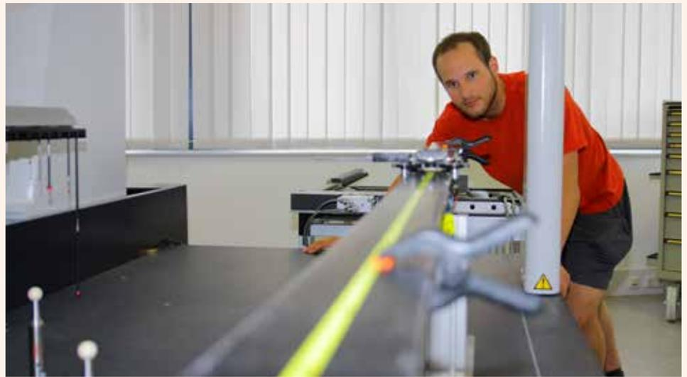
**Left:** Skis were positioned on the CMM using a mount for ski bindings.
